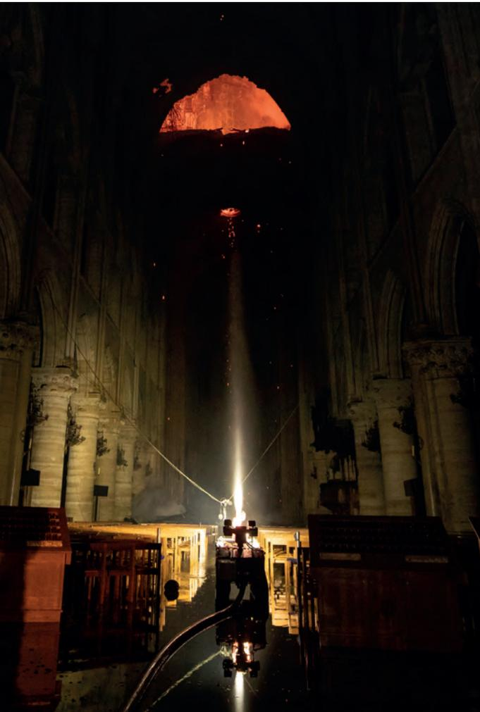
29. After dark the fire-fighting robot has been fighting for several hours the blaze in the nave after the collapse of the roof.
